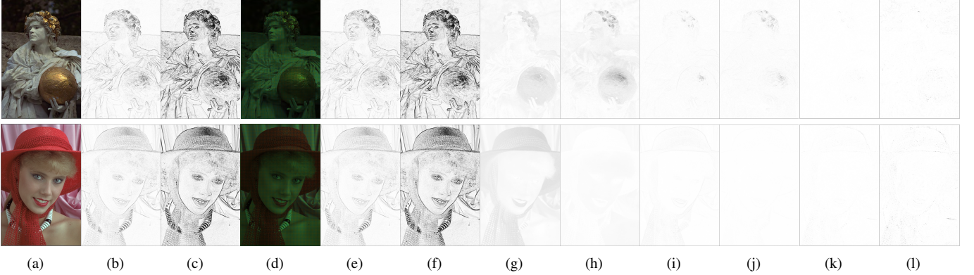
Fig. 6. Comparison of gradients extracted from color images and their Bayer version. (a) Image Kodim17 (top) and Image Kodim04 (bottom). (b)-(c): Gradient magnitude maps generated from (a) using the central difference operator and the Sobel operator in Fig. 2. (d) The resampled Bayer versions of Kodim17 and Kodim04 (displayed as a three-channel image). (e)-(f): Gradient magnitude maps generated from (d) using the central difference operator and the Sobel operator in Fig. 2. (g)-(h): The difference images generate from (a) by (G channel - R channel) and (G channel - B channel). (i)-(j): Gradient magnitude maps generated from (g) and (h) using operators in Fig. 2(a). (k) The gradient magnitude similarity (GMS) maps (29) between (b) and (e) with GMSD=0.004 (top) and GMSD=0.007 (bottom). (l) The GMS maps between (c) and (f) with GMSD=0.011 (top) and GMSD=0.022 (bottom).
