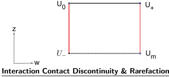
Figure 3: Interaction of a contact discontinuity with a rarefaction. The interacting waves are represented by FULL lines, a 2-wave or a 1-wave followed by a 1-wave. The dotted lines represent the resulting waves, a 1-wave (horizontal) followed by a 2-wave (vertical).
