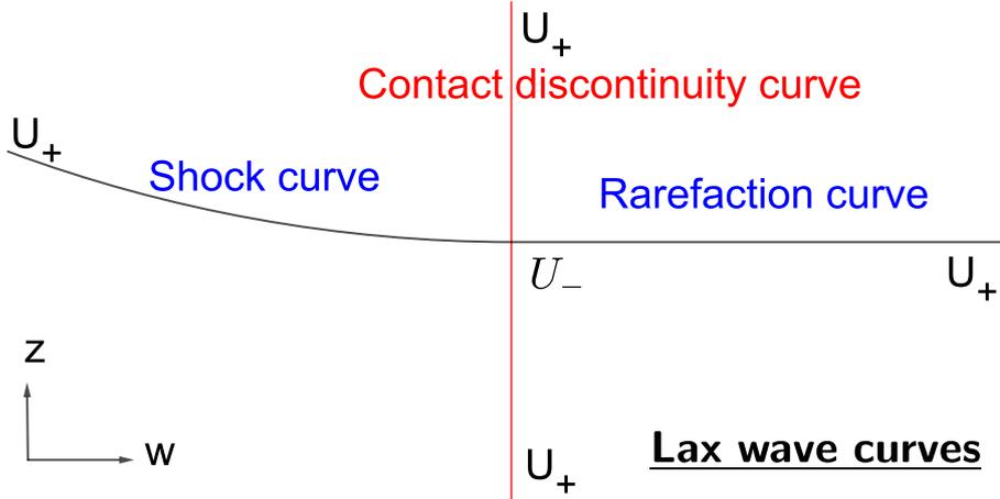
Figure 1: Lax waves curves where the state on the left of the wave  $U_- = (w_-, z_-)$  is fixed.  $U_+$  is the right state connected by a 1-wave when  $w$  varies,  $w_+ \neq w_-$ , or a 2-wave when  $w_+ = w_-$  is constant.
