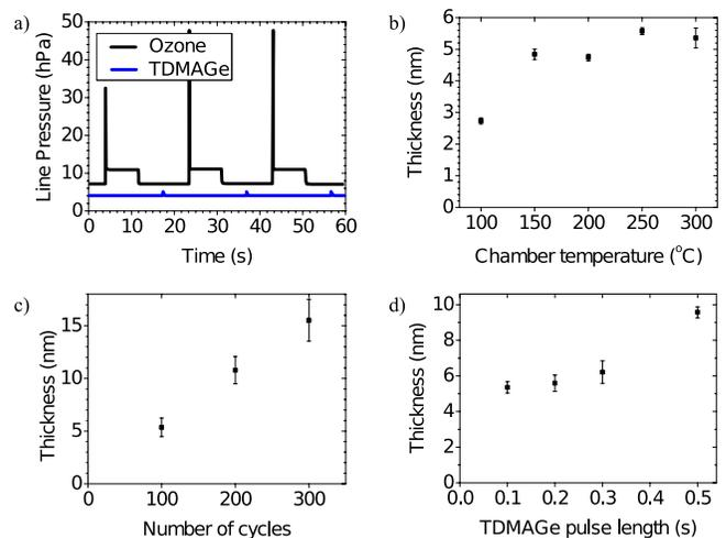
FIG. 2. a) Sketch of the pulse trains of the two precursors. b)  $GeO_2$  film thickness after 100 cycles at various reactor temperatures. c)  $GeO_2$  film thickness for different cycle numbers, at 300°C. A linear regression for this regime yields a GPC of 0.51Å. d)  $GeO_2$  film thickness for 100 cycles and at 300°C for different TDMAGe pulse lengths. Error bars are estimates based on sample dispersion.
