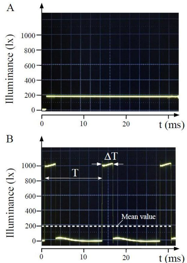
**Fig. 1.** The two lighting regimes. A) Target illuminance in the continuous regime. B) Target illuminance in the 80 Hz pulsed regime, with a duty cycle  $\Delta T/T = 0.2$ , to use the Hebbian mechanisms. The average illuminance is 200 lx in the two cases.
