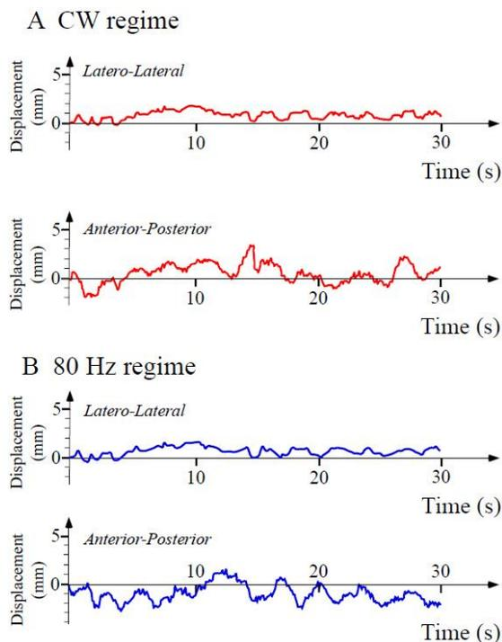
**Fig. 4.** Force platform results for a young adult without dyslexia. A) Latero-lateral and anterior-posterior variations under CW laboratory lighting. The surface of the stabilogram is  $10 \text{ mm}^2$ . B) Same results under 80 Hz pulse laboratory lighting. The results are unchanged (here the surface of the stabilogram is  $8 \text{ mm}^2$ ).
