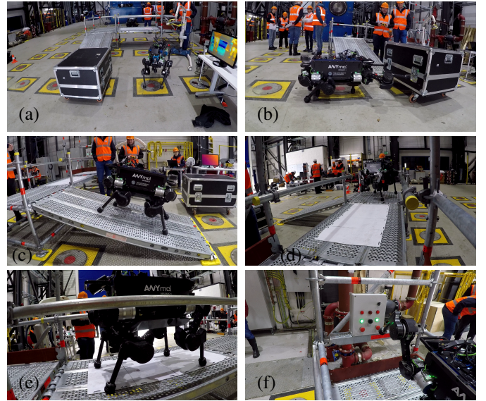
Fig. 8. Testing our system and algorithms in an industrial site: (a) starting from origin; (b) pushing the obstacle away; (c) climbing up on a 20^\circ slope; (d) turning around; (e) walking over slippery terrain; (f) teleoperating a foot to press E-stop.
