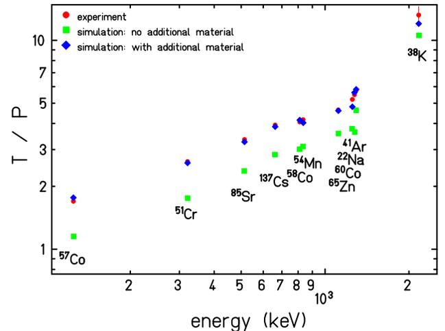
Fig. 2. Total-to-Peak ratio for  $\gamma$ -ray energies ranging from 122 keV to 2170 keV. The good agreement between experiment and simulation already obtained up to 1300 keV in our previous work is extended to 2170 keV.
