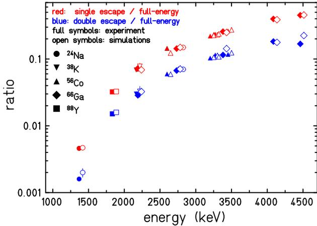
Fig. 3. Ratios of the single-escape (red) and double-escape (blue) intensities over the full-energy intensities from source measurements with  $^{24}\text{Na}$ ,  $^{38}\text{K}$ ,  $^{56}\text{Co}$ ,  $^{66}\text{Ga}$ , and  $^{88}\text{Y}$ . Full symbols represent experimental ratios, open symbols, slightly shifted to facilitate the reading of the figure, are from simulations with the CYLTRAN code. The additional point for  $^{38}\text{K}$  fits nicely in the systematics.
