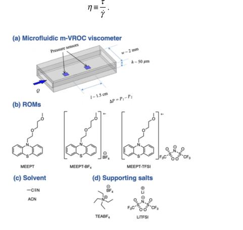
**Figure 1.** Representation of (a) microfluidic viscometer (image adapted from RheoSense Inc.), (b) ROMs: MEEPT (neutral), MEEPT-BF<sub>4</sub> (charged), and MEEPT-TFSI (charged), (c) solvent: acetonitrile (ACN), and (d) supporting salts: TEABF<sub>4</sub> and LiTFSI.
