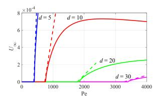
FIG. 5. Comparison of the results of numerical simulations (solid lines) with the predictions of asymptotic analysis, namely, Eq. (C25) (dashed lines) for  $D=10^{-3}$ ,  $\eta=1$ ,  $k_m=10$ ,  $k_r=1$ , and various swollen micelle sizes.
