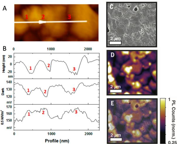
FIG. 3. (A) Topography map and (b) line profile data of topography and contact potential difference (CPD) under different conditions. (C) SEM, (D) fluorescence spectroscopy and (E) their composite image, showing that photoluminescence intensity spatially varies. Figures adapted with permission from Ref. 82 and 92.
