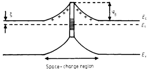
FIG. 2. A schematic one-dimensional band diagram of a grain boundary in an n-type semiconductor. The space-charge region is formed due to grain boundary states. Figure is adapted with permission from Reference 42.
