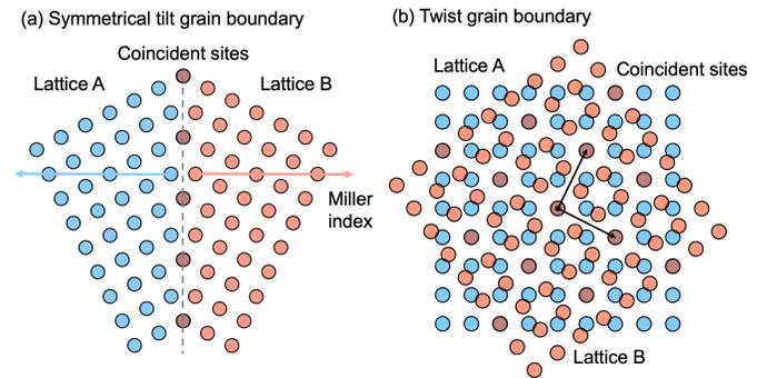
FIG. 1. Illustration of  $\Sigma 5$  (120) grain boundaries. (a) A symmetrical tilt grain boundary, and (b) a twist grain boundary. In (a), the boundary plane is denoted by a dashed line. In (b), the boundary plane is in between the two overlapped planes. Circles with different colors represent the lattice points of grains. When two neighboring lattices are expanded to the other side of the boundary, one of every five lattice points overlap, resulting in the  $\Sigma$  value of 5.
