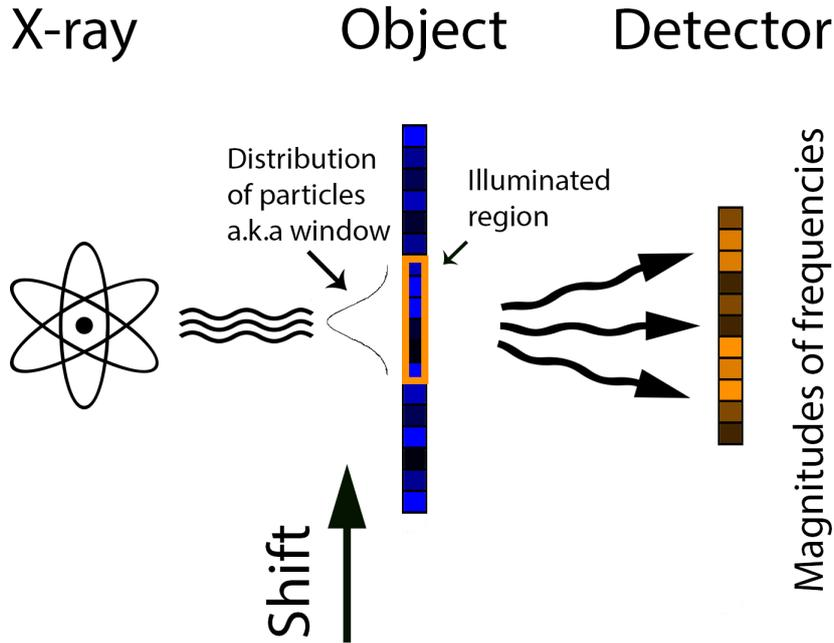
Figure 1: A typical one-dimensional ptychographic setup
