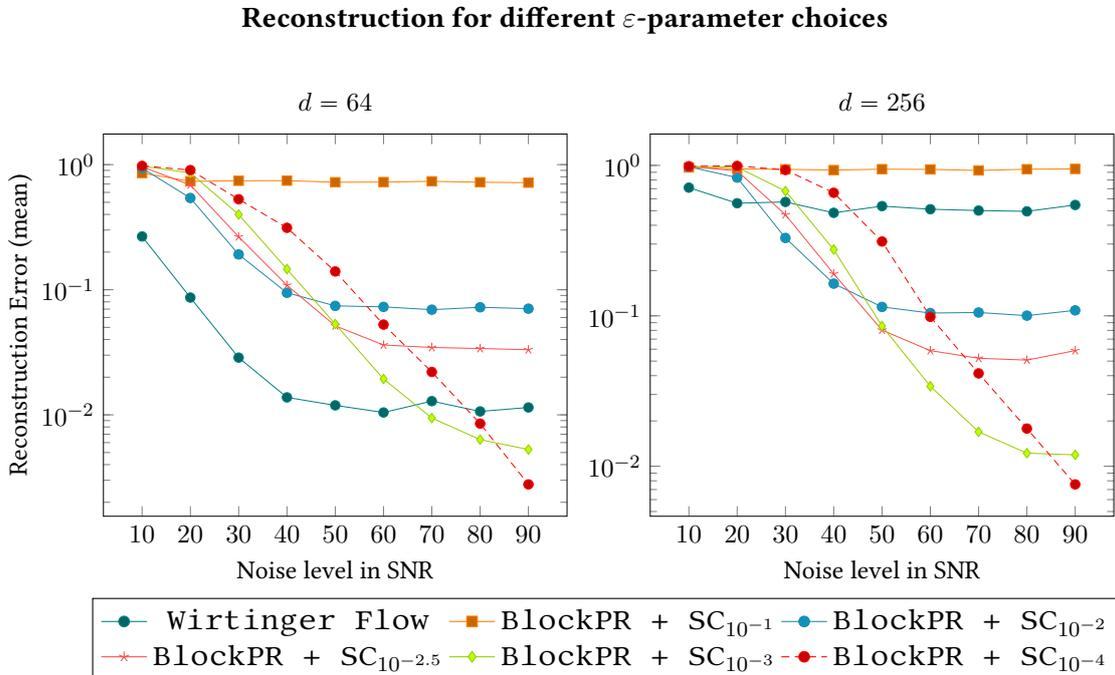
Figure 3: Comparison of the reconstruction accuracy for different truncation parameters  $\varepsilon$  for the *BlockPR* +  $SC_\varepsilon$  algorithm and *Wirtinger Flow* for window size  $\delta = 8$  and dimension  $d = 64$  (left) and  $d = 256$  (right).
