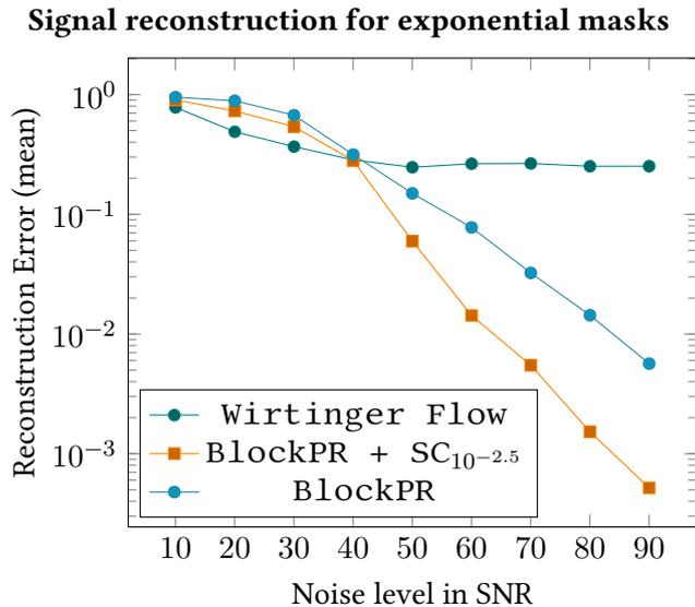
Figure 4: Reconstruction of a  $d = 64$  dimensional signal with exponential masks for *BlockPR*, *BlockPR + SC<sub>10<sup>-2.5</sup></sub>* and *Wirtinger Flow*
