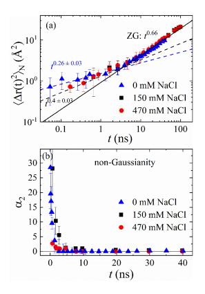
Figure 4. (a) The normalized mean squared displacement  $\langle \Delta r(t)^2 \rangle_N$  as a function of Fourier time, t, calculated from S(Q,t) for 0, 150 and 470 mM NaCl, dispersed in DOPC samples. The values for pure DOPC (0 mM) were taken from our previous study.<sup>27</sup> The solid and dashed lines represent the experimental power-law dependence. (b) The corresponding non-Gaussian parameters,  $\alpha_2(t)$ , as function of t.
