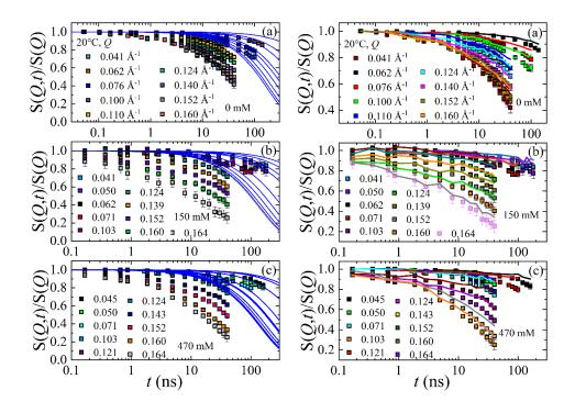
Figure 5. Influence of the translational diffusion of the vesicles on the dynamic structure factor, S(Q,t)/S(Q), for (a) 0, (b) 150, and (c) 470 mM NaCl. The solid lines (—) in the left column represent the calculation for translational diffusion,  $exp(-D_tQ^2t)$ , from low to high Q's (top to bottom). The solid lines in the right column represent experimental data divided by  $exp(-D_tQ^2t)$ . It highlights the deviation in the data introduced by the diffusion.
