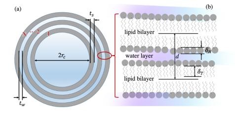
Figure 1. Schematic representation of (a) the multilamellar vesicle, and (b) lipid multilayers illustrating the number of bilayers, N, the radius of the core,  $r_c$ , the thickness of the individual shells,  $t_s$ , the thickness of the interleaved solvent layers,  $t_w$ , the thickness of the lipid head,  $\delta_H$ , the thickness of the lipid tail region,  $\delta_T$  and the lamellar repeat distance, d, of bilayers.
