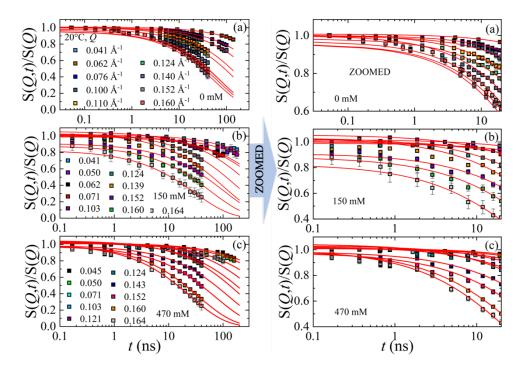
Figure 3. Dynamic structure factor, S(Q,t)/S(Q), as a function of Fourier time, t, for different Q's for DOPC in aqueous solutions with (a) 0, (b) 150, and (c) 470 mM NaCl. The solid lines (—) represent the ZG model (equation 10). Zoomed in right panel.
