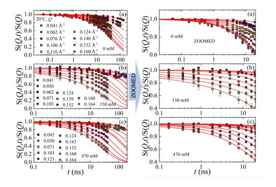
Figure 6. Dynamic structure factor, S(Q,t)/S(Q), as a function of Fourier time, t, for different Q's as indicated for (a) 0 mM (b) 150 mM, and (c) 470 mM NaCl samples. The solid (—) lines represent the model following the discussion in equation 9. Zoomed in right panel.
