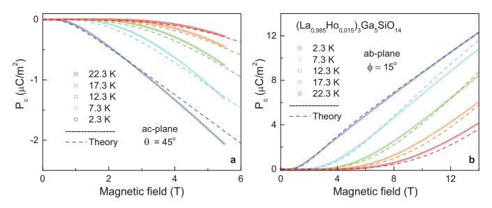
FIG. 3. Linear magnetoelectric effect in Ho-langasite. a. Electric polarization for fields in the *ac*-plane with  $\theta = 45^{\circ}$  (see also Fig. 2a). Solid lines are experimental data, dashed lines are results of theoretical calculations. b. Magnetic field dependence of the electric polarization,  $P_c$ , for applied magnetic fields rotated in the *ab* plane through 15° from the *b*\*-axis (see also Fig. 2b).
