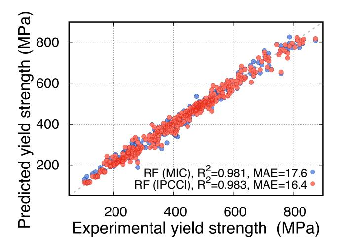
Figure 7 Experimental vs. predicted yield strength of the 9Cr steel with random forest (RF) with the top 10 features from both PCC and MIC analysis. MAE stands for mean absolute error (MAE).
