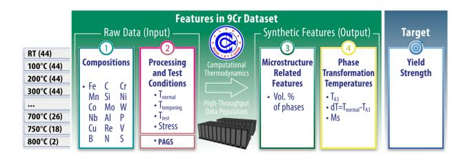
Figure 1 Alloy features considered in the 9Cr data analytics. Groups 1/2 are raw experiment data, and groups 3/4 are computed synthetic alloy features. This dataset cover data from room temperature to 800°C and the values in parentheses next to temperatures represent the number of data points at each temperature. Complete details of this dataset are reported in Table 1.
