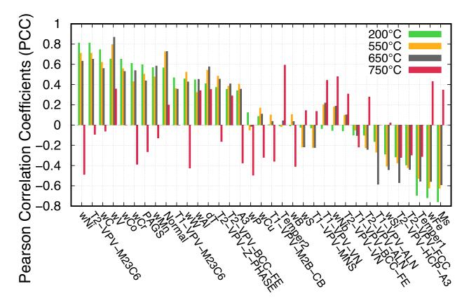
Figure 3 Results of correlation analysis between all features (composition, processing and test conditions, microstructure, and phase transformation temperature, see Table 1) and yield strength at selected representative temperatures. The correlation coefficients of the top 10 and bottom 10 features out of 45 features from 200°C (low temperature), 550 and 650°C (medium to high temperatures), and 750°C (above service temperature) are presented.
