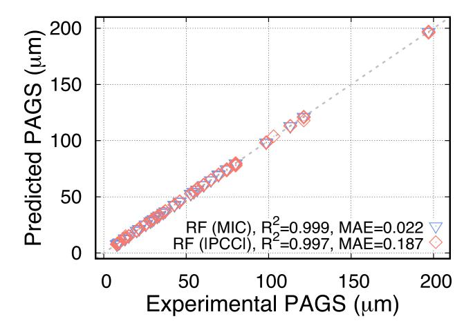
Figure 8 Experimental vs. predicted PAGS of the 9Cr steel with random forest (RF) with the top 10 features from MIC and PCC analyses. MAE stands for mean absolute error (MAE).
