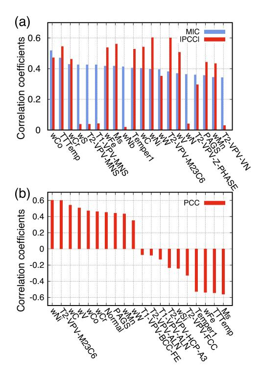
Figure 5 Correlation analysis between all alloy features and yield strength in the truncated ( $\leq 650^{\circ}$ C) dataset. (a) top 10 and bottom 10 features from the PCC analysis, and (b) top 20 ranking features from MIC and the corresponding features from |PCC|. The ranking of each feature from both analyses is reported in Table 2.
