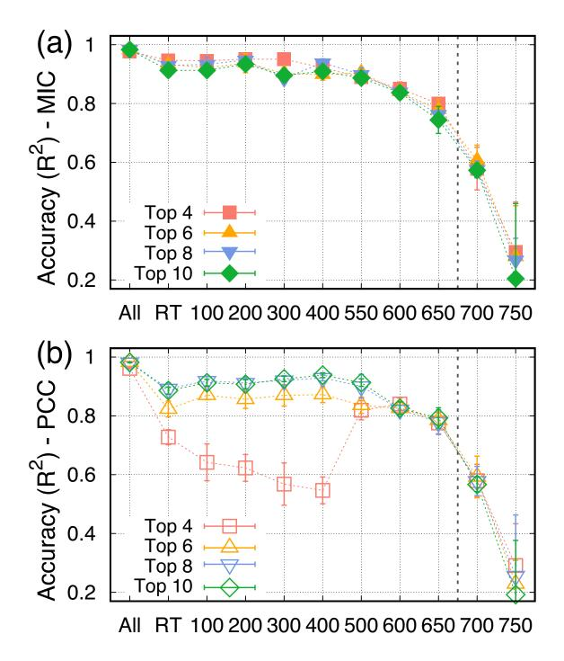
Figure 4 Accuracy of trained ML models (random forest as an example) as a function of temperature and numbers of top-ranking features from the (a) MIC and (b) PCC analyses. The models were trained for 10 times to determine the average accuracy and its standard deviation (error bar). The hyperparameters of each model were tuned up to 150 iterations to obtain optimum parameters. The vertical dash line indicates where issues of lack of data and relevant features start to occur.
