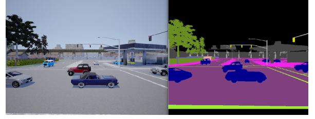
Fig. 4: CARLA frame showing raw and segmented camera images.
