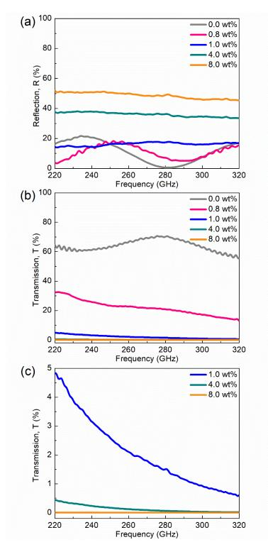
**Figure 2:** Coefficients of (a) reflection and, (b) transmission for composites with different graphene loadings in the 220 GHz – 320 GHz frequency range. (c) The lower bound of the transmission coefficient (T < 5%) allowing to distinguish the transmission coefficients for the composites with the graphene loading above 1 wt. %.
