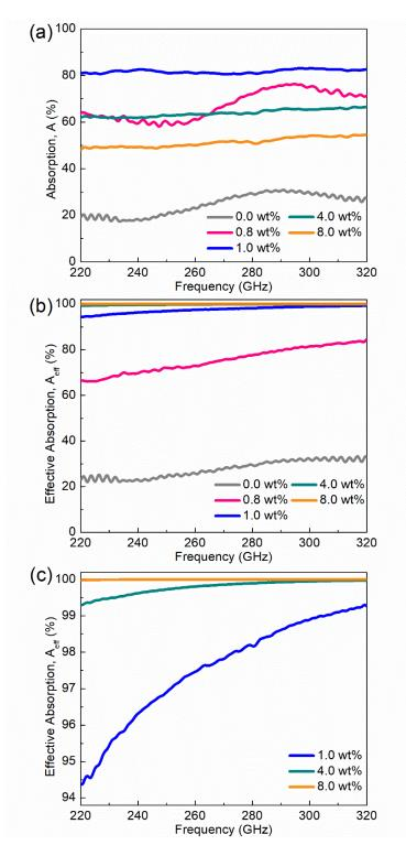
**Figure 3:** Coefficients of (a) absorption and (b) effective absorption for composites with different graphene loading fractions. (c) The upper bound of the effective absorption coefficient ( $A_{eff} > 95\%$ ) allowing to distinguish the values of  $A_{eff}$  for the composites with the graphene loading above 1 wt. %.
