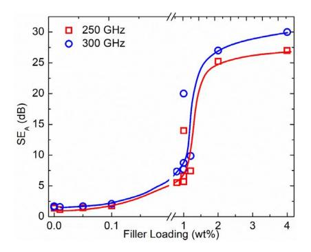
**Figure 5:** Absorption shielding efficiency as a function of graphene filler loading. Note an abrupt increase in  $SE_A$  at the filler loading, *f*, in the interval wt% < *f* < 2 wt%.
