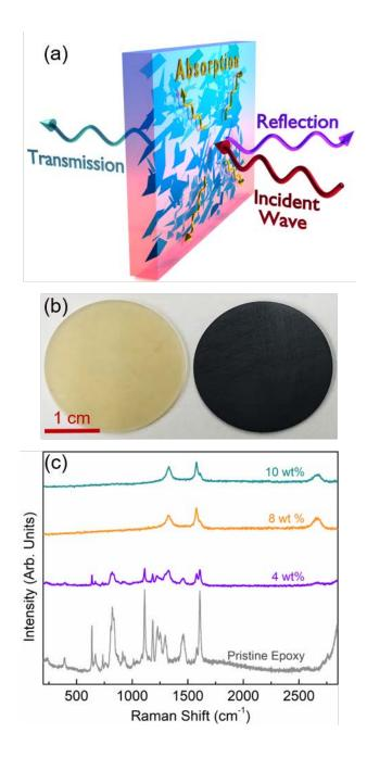
**Figure 1:** (a) Schematic of the interaction of the EM waves with the epoxy-based composites with the low filler loading of graphene. (b) Optical image of the pristine epoxy (left) and epoxy with f = 4 wt% of graphene (right). (c) Raman spectra of epoxy with different loading fractions of graphene fillers. Note the color change of the epoxy composite with addition of graphene. The composites can be used as adhessive for mouting microwave devices and as a coating layer.
