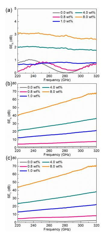
**Figure 4:** (a) Reflection  $(SE_R)$ , (b) absorption  $(SE_A)$ , and (c) total  $(SE_T)$  shielding efficiencies of composites at different graphene concentrations. As the filler loading increases,  $SE_R$  does not grow significantly wheras  $SE_A$  increasese substantially. The total shielding efficiency is substancially increased as a result of  $SE_A$  enhancement.
