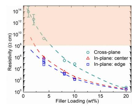
**Figure 6:** In-plane and cross-plane electrical resistivity of the samples as a function of graphene loading fraction measured at DC bias. The in-plane resistivity is smaller than that of the cross-plane direction, indicative that the fillers have preferential in-plane orientation as a result of the sample preparation procedures.
