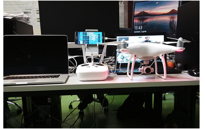
Fig. 8: The setup with Phantom 4, its RC, Android device, and GPU powered laptop.
