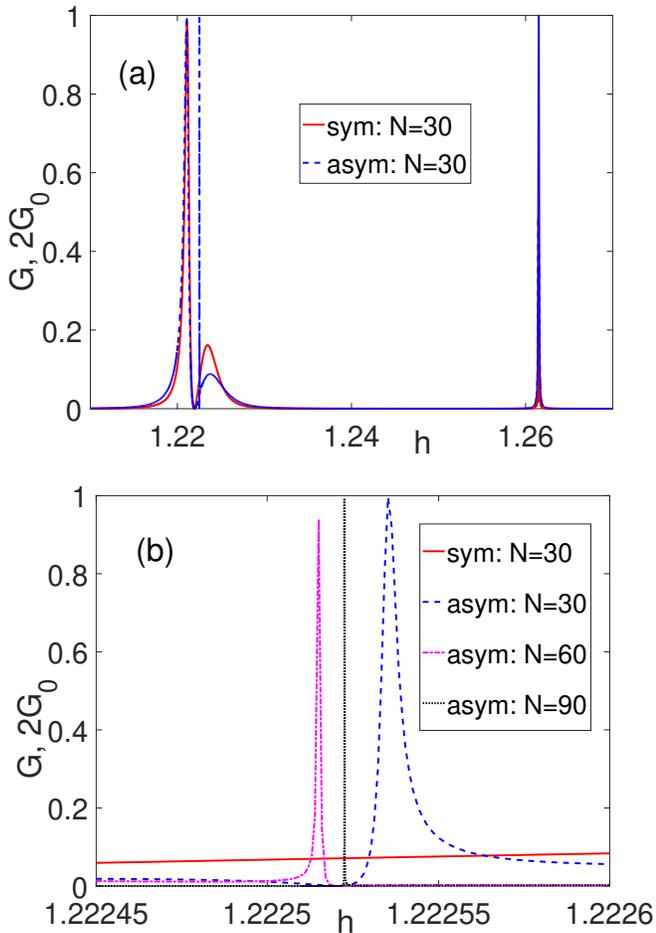
FIG. 3. Fig. 3. (a) Fano resonance arising due to the asymmetry of the tunneling processes in the ring. (b) Collapse of the Fano resonance illustrated in panel (a) with the increase in the degree of MS nonlocality. The values of parameters are  $n = 20$ ,  $N = 30$ ,  $t_0 = 0.1$ ,  $\epsilon_d = 1$ .
