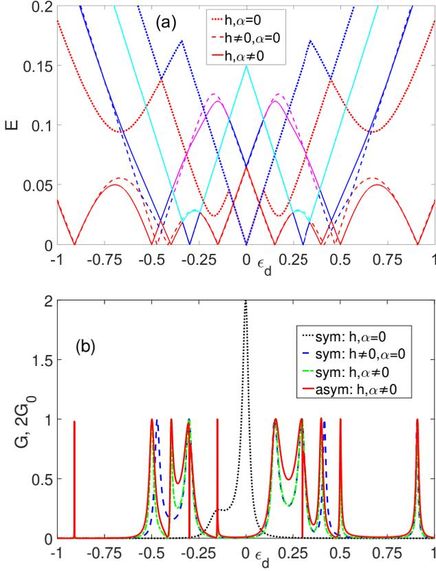
FIG. 2. Fig. 2. Excitation energies,  $E_{1-4}$ , ((a) and conductance (b) of the ring consisting of six sites versus electric field energy in the gate. Parameters:  $n = 1$ ,  $N = 2$ ,  $t_0 = 0.5$ ,  $h = 0.3$ .
