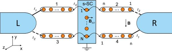
FIG. 1. Aharonov-Bohm ring with the arms connected by the superconducting wire exhibiting the Rashba spin-orbit coupling.
