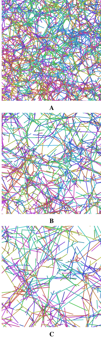
Figure 4: Visualization of slabs of 3PA meshes for networks with \langle N_{XK} \rangle = 10 ( A ), \langle N_{XK} \rangle = 35 ( B ), and \langle N_{XK} \rangle = 100 ( C ). Slabs and chain colors as in Fig. 3
