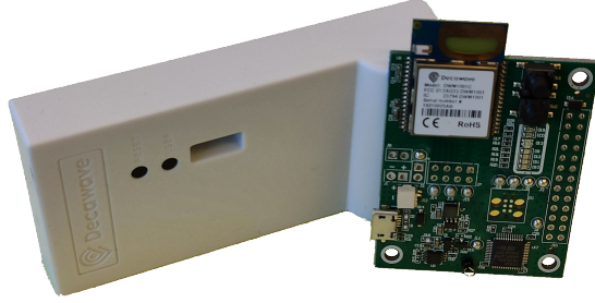
Fig. 2: Decawave's DWM1001 Development Board, which has been utilized in the experiments
