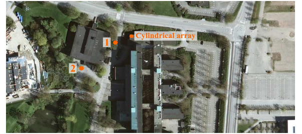
Fig. 2: The outdoor scenario for both LOS (position 1) and NLOS (position 2). The base station has a cylindrical array and is positioned on the roof. The users were moving within a circle with a diameter of 5 m.
