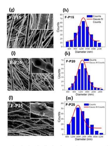
Figure 2. SEM images and grain size distribution for PZT/PVDF composites with different PZT: (a-b) 0 wt%, (c-d) 5 wt%, (e-f) 10 wt%, (g-h) 15 wt%, (i-k) 20 wt%, (l-m) 25 wt%.
