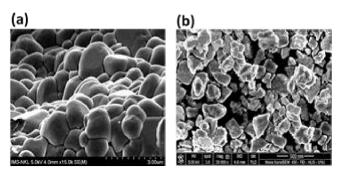
Figure 1. SEM images of particle size of the PZT before and after grinding
