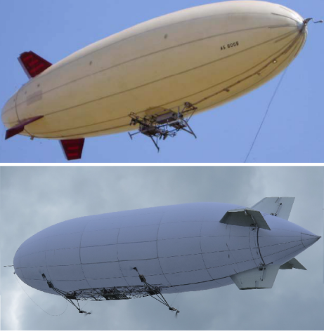
Fig. 1: Top: pioneer AURORA airship used in different research investigations. Bottom: NOAMAY airship platform (2018), whose flight simulator is used in this work.
