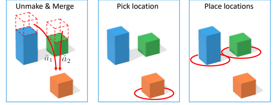
Fig. 3: The proposed unmake procedure disassembles objects in multiple ways (left) and generates set of pick & place actions available from each state (right). For visual policies, we use the heatmap representation to predict all the actions simultaneously.
