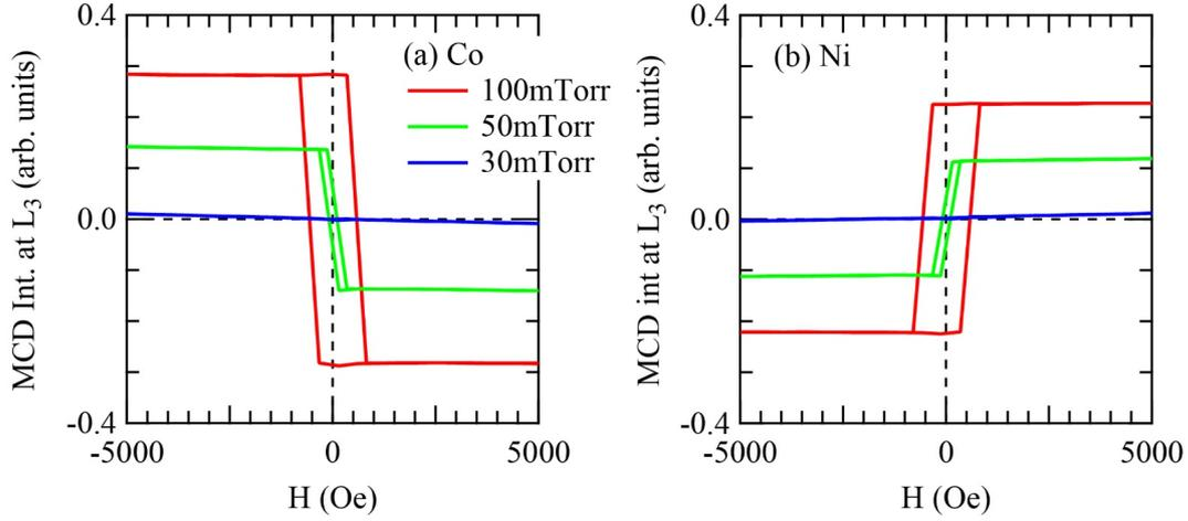
Figure 3: Magnetic field dependence of (a) Co  $L_3$ - and (b) Ni  $L_3$ -XMCD peak intensity for NCO films grown under  $P_{O_2} = 30, 50$  and  $100\text{mTorr}$ . The data were collected in the  $\theta_H=0^\circ$  configuration and with the incident x-ray energy fixed to be  $779.0\text{eV}$  for the Co  $L_3$ -XMCD signal and  $853.5\text{eV}$  for the Ni signal.
