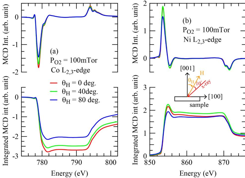
Figure 4: (a) Co  $L_{2,3}$ - and (b) Ni  $L_{2,3}$ -XMCD spectra and their integrated intensity for the  $P_{O_2} = 100$ mTorr film. The spectra were measured with the magnetic field angle  $\theta_H$  of 0, 40, and 80 degrees. The measurement configuration is shown in the inset of the figure.
