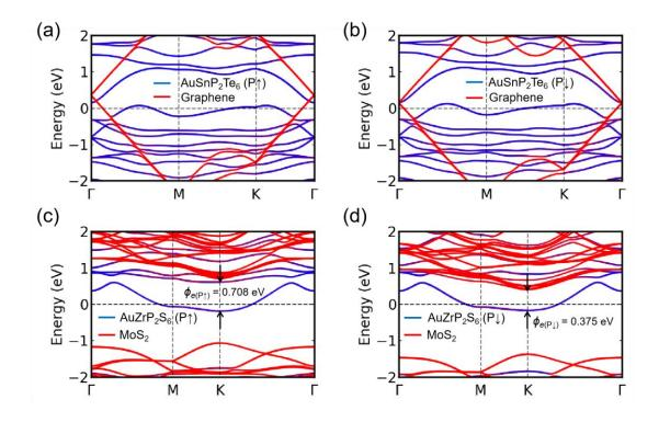
**Fig. 5.** Band structures of heterostructures. (a, b)  $AuSnP_2Te_6/Graphene.$  (c, d)  $AuZrP_2S_6/MoS_2$ . The directions of polarization (*P*) in ferroelectric metals are marked by black thin arrows. The blue and red colors indicate the contributions from different 2D materials.
