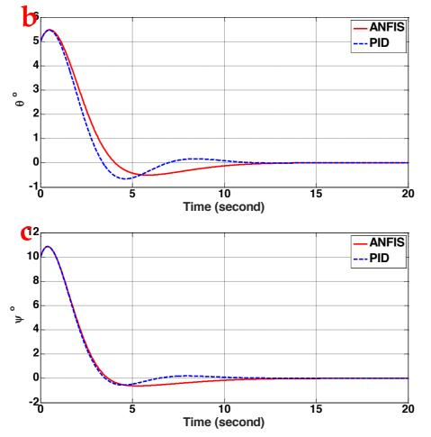
**Figure 10.** Comparison of Euler angles (a)  $\varphi$  (b)  $\theta$  and (c)  $\psi$  using ANFIS and PID controller in presence of uncertainty.
