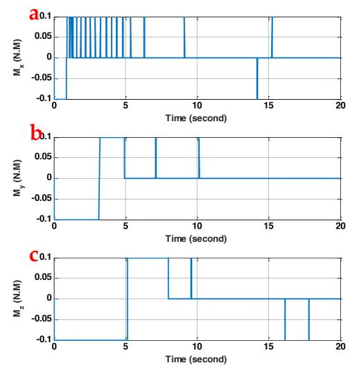
Figure 12. The control moment of Thruster in (a) X, (b) Y, and (c) Z axis.
