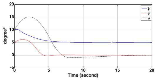
**Figure 11.** Euler angles time history using PWPF modulator
