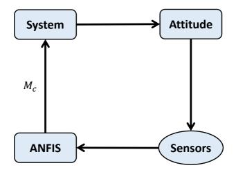
Figure 6. Block diagram of control system using ANFIS integrated controller and observer.
