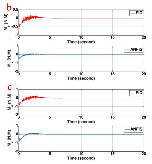
Figure 7. Comparison of control moment in (a) X (b) Y and (c) Z directions using ANFIS and PID in presence of noise.
