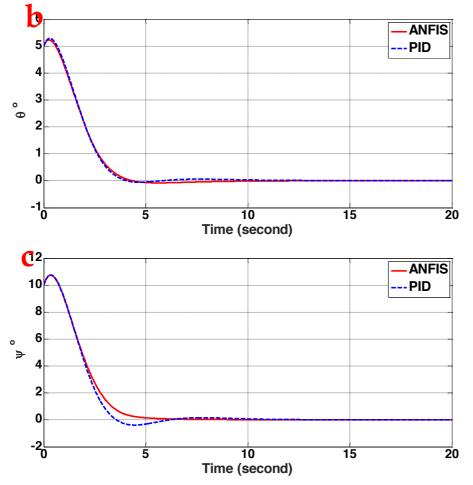
**Figure 8.** Comparison of Euler angles (a)  $\varphi$  (b)  $\theta$  and (c)  $\psi$  using ANFIS and PID controller in presence of noise.
