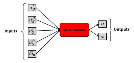
Figure 3. Block diagram of ANFIS observer.
