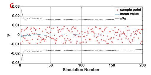
**Figure 13.** Monte-Carlo simulation error for (a)  $\varphi$ , (b)  $\theta$ , and (c)  $\psi$ .
