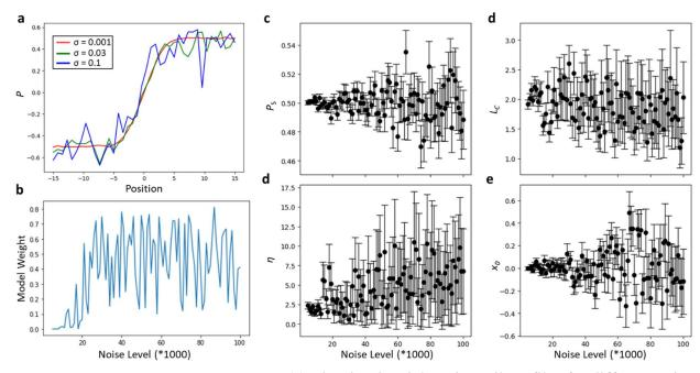
**Figure 6. Noise and sampling effects.** (a) The simulated domain wall profiles for different noise levels. (b) Weight of Model 1 and 2 comparison of WAIC scores versus input noise. Zero value corresponds to correct identification of the wall type. (c-e) The extracted parameters from the Bayesian inference fits for single realization of the synthetic data set versus input noise.
