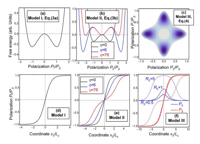
Figure 1. LGD ferroelectric domain wall models. (a, b, c) Free energy vs. order parameter – polarization components  $P_i/P_S$  and (d, e, f) distribution of these  $P_i/P_S$  across the domain wall for Models 1-3. Note that we fixed the coefficients  $a_1$ ,  $a_{11}$  and  $a_{111}$ , and recalculated the spontaneous polarization  $P_S$  and parameter  $\eta$  from them for Model 2. For Model 3, component  $P_1$  is not observable by STEM.
