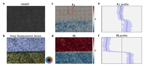
Figure 4. Experimental data for 180° domain wall. (a) HAADF-STEM subregion of  $180^{\circ}$  BiFeO<sub>3</sub> domain wall. (b) Cation displacement vector map. (c) Color-scaled lattice positions of the **P** component perpendicular ( $[\bar{1}01]_{pc}$  axis) and (d) parallel ( $[101]_{pc}$  axis) to the domain wall. (e) Profiles of the mean values (datapoints) and 90% data bounds (blue) for perpendicular and (f) parallel **P** components.
