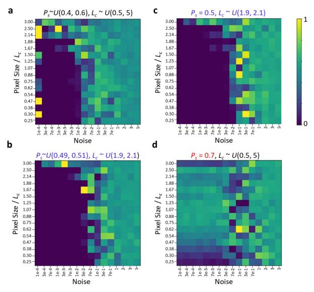
Figure 7. Effect of prior knowledge on imaging required for model separation. Matrices show the weight for WAIC score comparisons of Models 1 and 2 against synthetic domain wall data as a function of the effective pixel size and noise level. Universal color scalebar is at right of the image, 0 corresponds to models being reliably separated, 0.5 is indistinguishable, and 1 is incorrect inference. The true value of parameters are  $x_0 = 0$ ,  $P_s = 0.5$ ,  $L_c = 2$ , and  $\eta = 2$ . The prior
