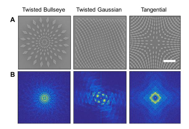
**Figure 2.** Aperiodic metasurfaces investigated in this work. (A) SEM micrographs of the experimentally fabricated Twisted Bullseye, Twisted Gaussian, and Tangential aperiodic arrays, together with their diffraction patterns calculated by FFT (B). The scale bar corresponds to 500 nm and applies to all images in (A).
