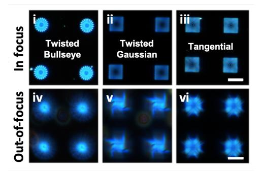
Figure 3. Far-field response of the aperiodic metasurface patterns. Optical dark field images in- and out-of focus (with focus of ca. 3  $\mu$ m away from the surface) recorded from arrays of the three functional patterns. The far-field modulation of the plasmonic patterns is manifested in the out-of-focus images by a vortex for the TBE and Twisted Gaussian patterns, and by the 4 leaf-clover like light distribution for the Tangential pattern. Scale bars are 5  $\mu$ m and apply to all images.
