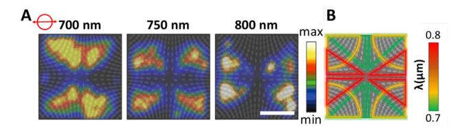
Figure 7. Tangential pattern: Wavelength induced rotation of the near-field distribution. (A)
