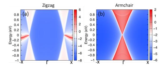
FIG. 7 Edge states of zigzag (a) and armchair (b) graphene ribbons without considering the SOC effect. For the armchair edge, the two Dirac points in the bulk system project onto the same point, thus, there is only one Dirac point for the armchair ribbon.
