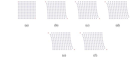
**Figure 8.** FNI interacting system subject the pulling of two opposite vertices in opposite horizontal directions. Actual configurations for six instants of time are plotted: (a) t = 1; (b) t = 100; (c) t = 200; (d) t = 300; (e) t = 400; (f) t = 500.
