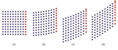
**Figure 4.** SNI system subject to shear external action: the right side (in red) is pulled in the positive y direction, the left side is clamped. Actual configurations for four instants of time are plotted: (a) t = 1; (b) t = 30; (c) t = 60; (d) t = 90.
