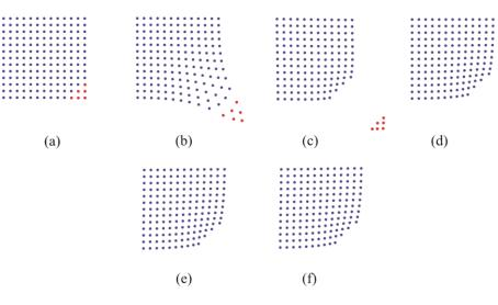
**Figure 14.** Parametric study of fracture: in this figure the behaviour of the system for < 11 is shown. Actual configurations for six instants of time are plotted: (a) t = 1; (b) t = 30; (c) t = 60; (d) t = 90; (e) t = 120; (f) t = 150.
