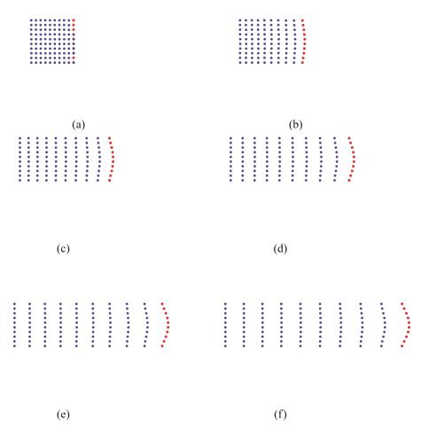
**Figure 10.** FNI system with the left side clamped and the right one pulled horizontally in the positive x direction. Actual configurations for six instants of time are plotted: (a) t = 1; (b) t = 60; (c) t = 120; (d) t = 180; (e) t = 240; (f) t = 300.
