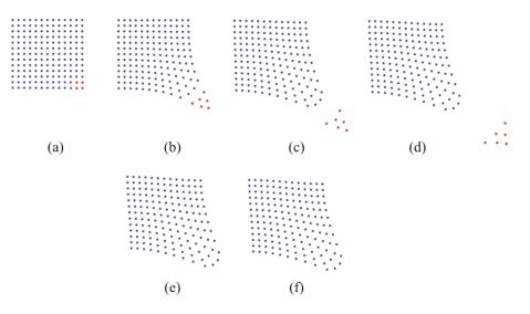
**Figure 15.** Parametric study of fracture: in this figure the behaviour of the system for >11 is shown. Actual configurations for six instants of time are plotted: (a) t = 1; (b) t = 30; (c) t = 60; (d) t = 90; (e) t = 120; (f) t = 150.
