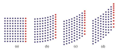
**Figure 3.** FNI system subject to shear external action: the right side (in red) is pulled in the positive y direction, the left side is clamped. Actual configurations for four instants of time are plotted: (a) t = 1; (b) t = 30; (c) t = 60; (d) t = 90.
