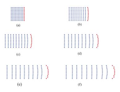
**Figure 11.** SNI system with the left side clamped and the right one pulled horizontally in the positive x direction. Actual configurations for six instants of time are plotted: (a) t = 1; (b) t = 60; (c) t = 120; (d) t = 180; (e) t = 240; (f) t = 300.
