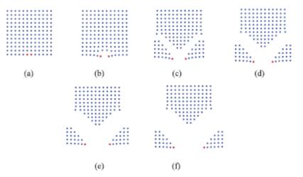
**Figure 17.** System subject to the pulling of two central elements of the bottom side. The left leader is pulled in the (-1, -1) direction, the right one in the (1, -1). Actual configurations for six instants of time are plotted: (a) t = 1; (b) t = 40; (c) t = 80; (d) t = 120; (e) t = 160; (f) t = 200.
