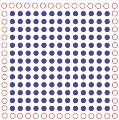
**Figure 2.** Graphical representation of fictitious elements. Every fictitious element (empty dots) translates rigidly with the closest true element. The vertex true elements carry in rigid translation the vertex fictitious element and its two fictitious neighbours.
