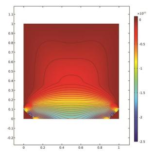
**Figure 19.** Level lines of compressive principal stress direction (and the relative eigenvalue in the color map) in the case of continuum finite element simulation with an imposed displacement similar to the one considered in the previous discrete simulation.
