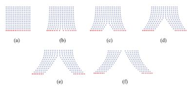
**Figure 13.** System subject to the pulling of two halves of the bottom side in opposite directions. Actual configurations for six instants of time are plotted: (a) t = 1; (b) t = 48; (c) t = 96; (d) t = 144; (e) t = 192; (f) t = 240.
