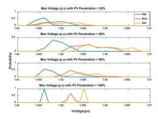
Fig. 10. Maximum voltage probability for optimal, random, 10 kW standard PV allocation methods
