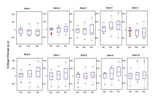
Fig. 13. Zonal voltage change (30-min data resolution)
