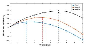
Fig. 5. Optimal PV sizes for three houses
