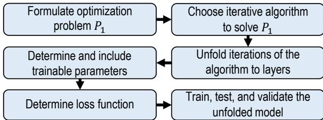
Fig. 3: Methodology for Deep unfolded signal processing
