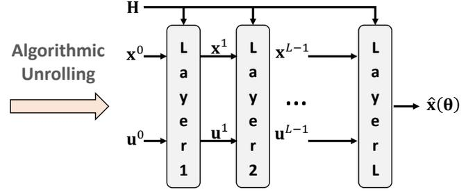
Fig. 4: Deep unfolded representation of ADMM-Net
