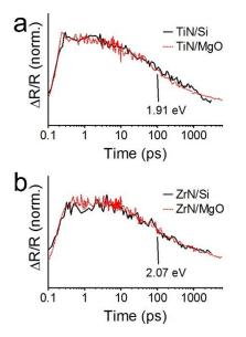
Figure S7. Normalized transient reflectivity under 3.89 eV pump photon energy excitation of (a) films of TiN on silicon and MgO and (b) films of ZrN on silicon and MgO. The probe
