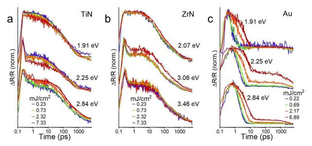
Figure S4. Fluence-dependent dynamics for 3.1 eV pump photon energy excitation of (a) TiN and (b) ZrN films on silicon and (c) Au film on silicon. Data are shown for selected probe energies shown on right. Solid fit lines are overlaid on the data.
