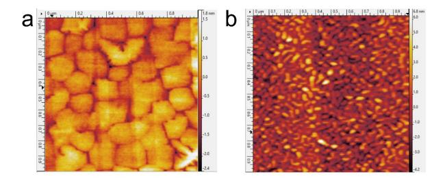
Figure S2. Atomic force microscopy contour plots of (a) TiN and (b) ZrN films on MgO.
