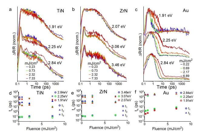
Figure 3. Normalized, fluence-dependent transient reflectivity with 3.1 eV pump photon energy for (a) TiN on MgO, (b) ZrN on MgO, and (c) Au on silicon. (f) Triexponential fit results for the data collected on TiN as a function of fluence. (e) Triexponential fit results for data collected on ZrN as a function of fluence. (f) Biexponential fits results for the data collected on Au as a function of fluence at the specified wavelengths.
