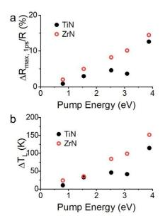
Figure 5. (a) Maxima of transient reflectivity spectra versus pump photon energy. (b) Estimated temperature rise of the samples under the given excitation conditions. Except for 0.80 eV (12 mJ/cm<sup>2</sup>), the pump fluence was kept at 2.3-2.4 mJ/cm<sup>2</sup>.
