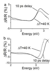
Figure S9. (a) Raw differential reflectivity data of TiN film on MgO from static thermoreflectance measurements (dashed) with a temperature difference of 40 K (starting from 295 K) and the transient reflectivity spectrum at 10 ps delay for the same film with 3.1 eV photon excitation. (b) analogous data for ZrN film on MgO.
