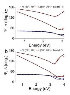
Figure 12. Raw spectroscopic ellipsometry results ( $\Psi$  and  $\Delta$ ) shown in solid lines of blue and red, respectively, with a dashed line showing the model fit of the data for (a) TiN on MgO and (b) ZrN on MgO.
