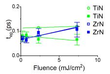
Figure S5. Linear fits to electron-phonon coupling time constant ( $t_{ep}$ , symbols) with variable fluences. Open symbols represent the higher probe and closed symbols the lower probe energy. Data from Figures 3 and S4. The y-intercept is taken as the fundamental electron-phonon coupling time constant of the material.
