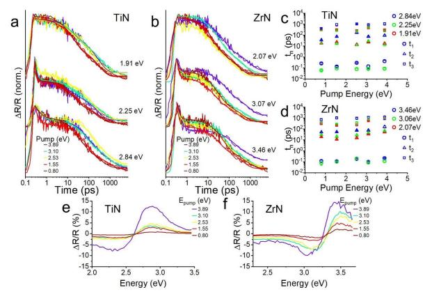
Figure S11. Dynamics of (a) TiN and (b) ZrN films on MgO for specified pump photon energies, measured at probe wavelength specified at right on plots. Solid fit lines are overlaid on data. Fit results for (c) TiN and (d) ZrN are shown in the scatterplots. Spectra of (e) TiN and (f) ZrN at 1 picosecond delay for specified pump photon energies. Except for 0.80 eV (12 mJ/cm<sup>2</sup>), the pump fluence was kept at 2.3-2.4 mJ/cm<sup>2</sup>.
