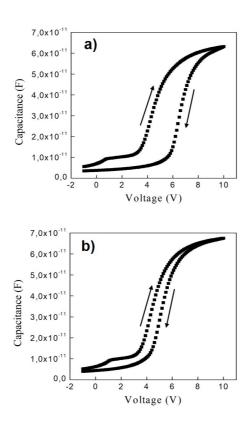
FIG. 5. C-V curves, recorded at 1 MHz, of Al<sub>2</sub>O<sub>3</sub>/HfO<sub>2</sub> nanolaminated films asdeposited by PE-ALD (a) and after annealing process at 800°C in N<sub>2</sub> atmosphere (b).
