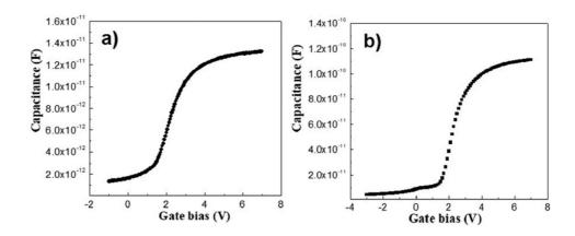
Fig. 3. C/V curves recorded at 1 MHz for  $Al_2O_3$  (a) and  $HfO_2$  (b) films deposited by PE-ALD processes.
