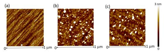
FIG. 2. AFM bidimensional maps of the SiO<sub>2</sub>/4H-SiC substrate (a), Al<sub>2</sub>O<sub>3</sub> (b) and HfO<sub>2</sub> (c) thin films grown by PEALD processes.
