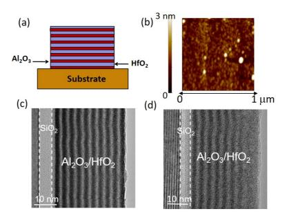
FIG. 4. Schematic of the  $Al_2O_3/HfO_2$  laminated film (a) and its AFM bidimensional map (b). The cross section TEM image (c) shows the formation of about 1.8 nm alternating  $Al_2O_3$  and  $HfO_2$  thin layers in the as-dep film, whose interfaces became not so defined after annealing, as shown in the TEM image (d) recorded after the  $800^{\circ}C$  treatment.
