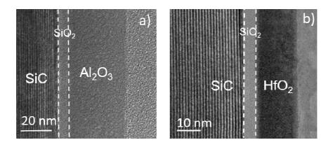
Fig. 1. TEM cross-section images of  $Al_2O_3$  (a) and  $HfO_2$  (b) thin films grown by PEALD on  $SiO_2/(0001)$  SiC substrates.
