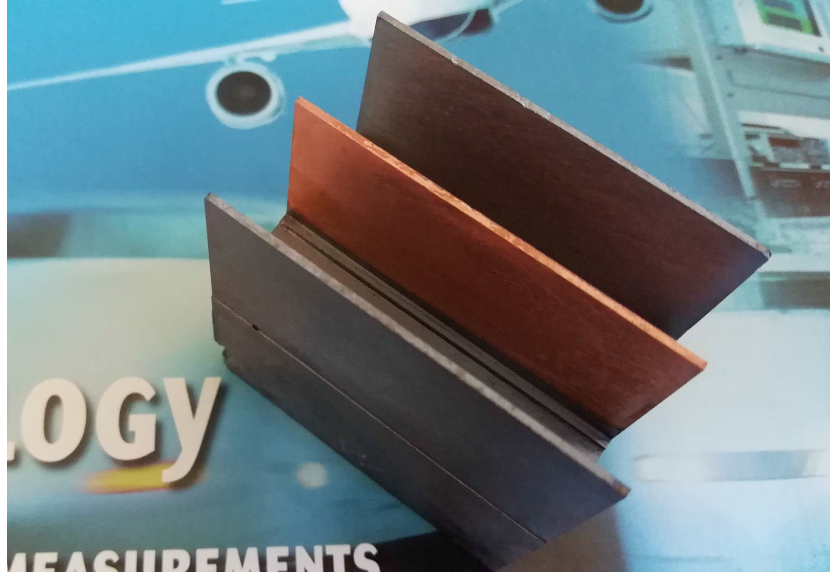
Figure 2: Photograph of the x-ray interferometer with a Cu film on the mirror crystal. The film thickness has been increased to make it visible.
