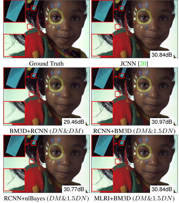
Figure 4: Demosaicking and denoising results on an image from the Kodak dataset with \sigma = 20 . We compare an DN\&DM scheme BM3D+RCNN [14], with three DM\&1.5DN RCNN+CBM3D, RCNN+nlBayes and MLRI+BM3D. As a reference we also include the result of a joint CNN method JCNN [20]. But its results are only available for noise with \sigma \leq 20 because the network is not trained beyond that level.
