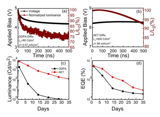
**Figure 4.** Luminance and driving voltage for (a) ODPA capped DiR LED and (b) AET capped DiR LED *versus* operating time under ambient conditions. Note the much higher driving current density and luminance (66 mA/cm<sup>2</sup> and 500 cd/m<sup>2</sup>, respectively) in the case of AET with respect to ODPA (0.07 mA/cm<sup>2</sup> and 95 cd/m<sup>2</sup>). (c-d) Luminance (c) and EQE (d) versus shelf time for ODPA and AET based devices.
