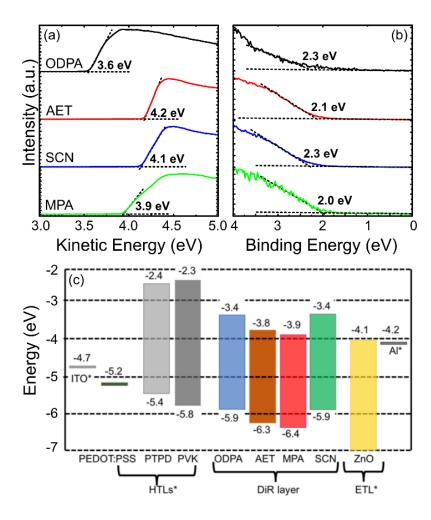
**Figure 3.** (a, b) UPS spectra obtained from the different DiR films. (c) Flat-band diagram of the LED structure. The energy bands of the differently functionalized DiR films are shown side-by-side for ease of comparison, however, only one layer is implemented in the LED at a time.
