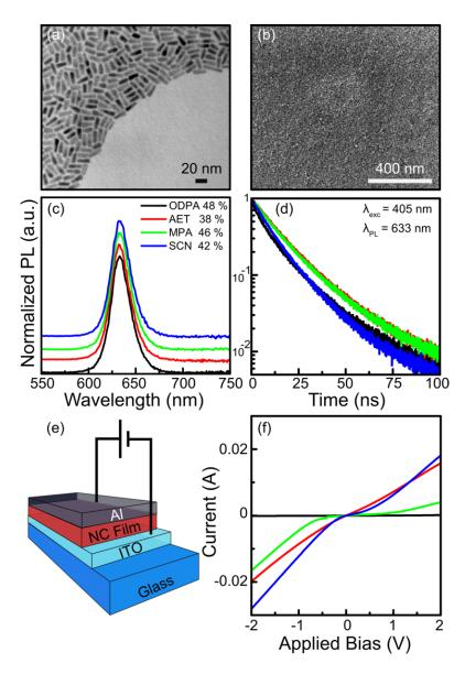
Figure 1 (a) Transmission electron microscope (TEM) image of CdSe/CdS Dot-in-Rods (average length = 17 nm, width = 9 nm and CdSe core diameter = 4.3 nm). (b) Scanning electron microscope
