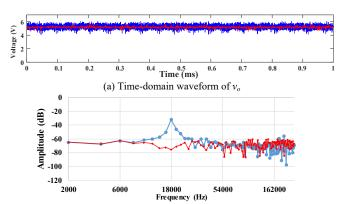
(b) Normalized frequency spectrum of  $v_0$ Fig. 18. Time-domain waveform and normalized frequency spectrum of  $v_o$  of the two-stage wireless power receiver without frequency synchronization (in blue) and with frequency synchronization (in red).
