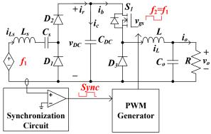
Fig. 13. Two-stage wireless power receiver using frequency-synchronized buck converter.
