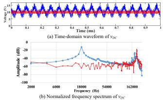
Fig. 17. Time-domain waveform and normalized frequency spectrum of  $v_{DC}$  of the two-stage wireless power receiver without frequency synchronization (in blue) and with frequency synchronization (in red).
