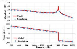
Fig. 8. Bode plots of small-signal response of  $\Delta V_{o<0>}$  to  $\Delta d$
