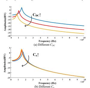
Fig. 11. Plots of the normalized beat frequency oscillation  $V_{DC < MI-M2}$  versus beat frequency at different  $C_{DC}$  and  $C_o$ .
