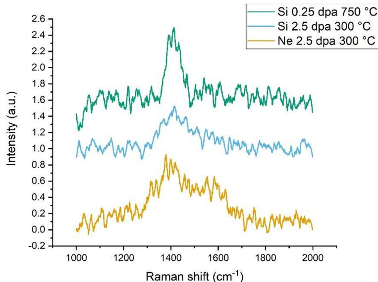
Figure 4: Spectra from the C-C bonding region of irradiated 6H-SiC with a straight baseline subtraction. The silicon irradiated samples have a single peak at  $\sim 1410\text{ cm}^{-1}$  while the neon irradiated sample has a double peak at  $1400\text{ cm}^{-1}$  and  $1580\text{ cm}^{-1}$ .
