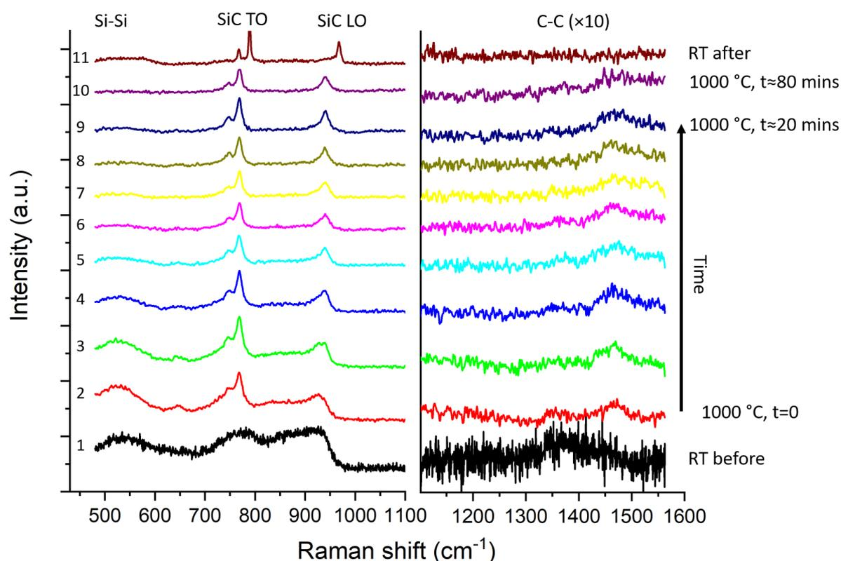
Figure 5: Raman spectra of 6H-SiC acquired during annealing at 1000 °C in air. “Before” and “After” lines were measured at room temperature using the same  $\times 50$  long focal length objective and heating stage window as the high temperature spectra. The C-C region of the spectra are magnified  $\times 10$  to see these low intensity peaks more clearly.
