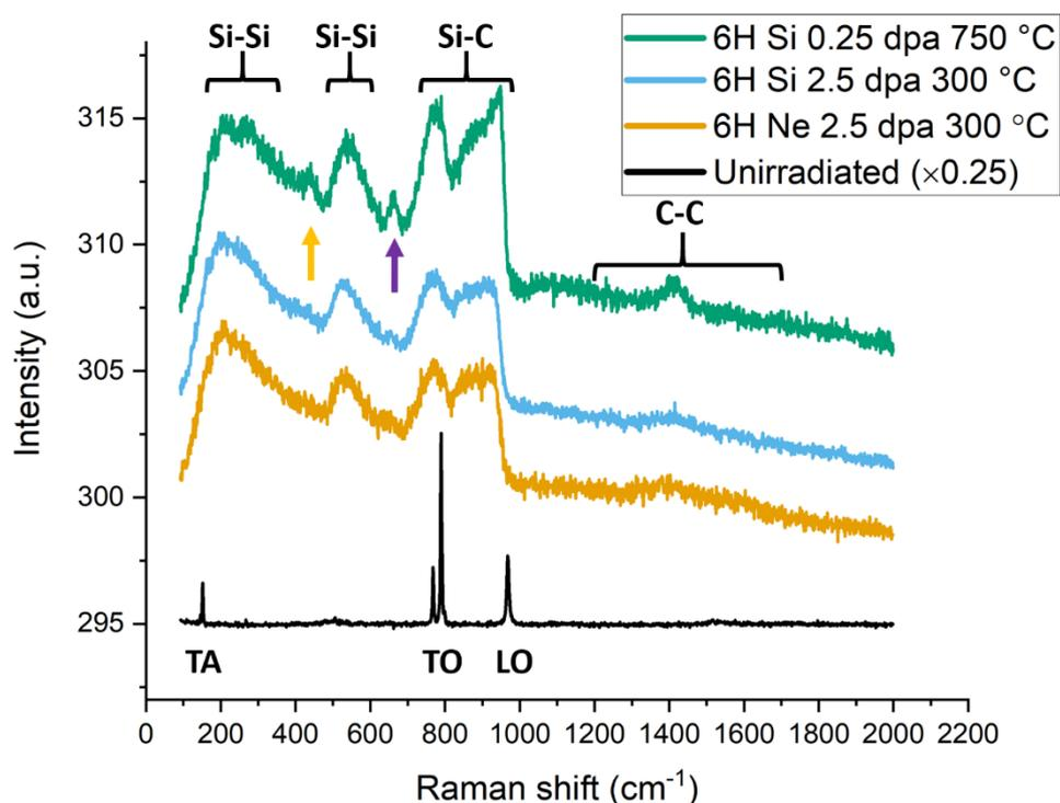
Figure 3: Raman spectra of unirradiated and ion implanted single crystal 6H-SiC. The unirradiated spectrum is multiplied by  $\times 0.25$  in the y axis and is from the unirradiated region of the 750 °C irradiated specimen. Orange arrow points at a peak for Si-O-Si bonding, and the purple arrow to C-O-C bonding.
