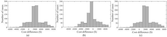
Fig. 8: Histogram of cost difference (cost<sub>ESCUC-expected</sub> - cost<sub>ESCUC-base</sub>) of the pairs: (a) base-case costs (b) original expected costs (c) realized N-1 costs.
