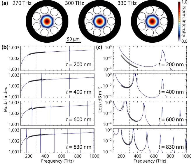
**Fig. 1.** (a) Structure of the single-ring PCF (50  $\mu\text{m}$  core diameter, 400 nm capillary wall thickness, filled with 10 bar argon) and intensity distribution of the fundamental core mode at frequencies of 270, 300 and 330 THz. (b) Modal index [20] and (c) loss [21] of the fiber, for capillary wall thicknesses  $t = 200, 400, 600$  and  $830$  nm. The gray dots are data from finite element modelling. The dashed lines denote the pump frequency used in this work (300 THz).
