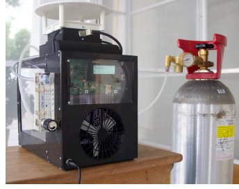
Fig. 10 Smart Trap for counting and classifying mosquitoes in real-time using optical sensor.
