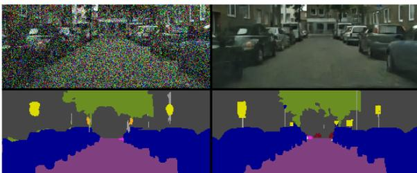
Figure 5: Dense UMC results for noisy images  $\sigma = 60$ . Top row, left to right: input noisy image, denoised image; bottom row, left to right: segmentation prediction, segmentation ground truth
