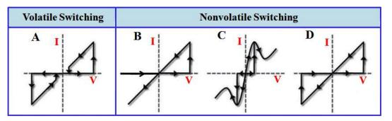
Fig.2. Schematic of the I-V characteristics for the volatile and non-volatile switching devices - A) volatile Threshold switching, B) WORM switching, C) unipolar switching and D) bipolar switching behaviour [reprinted with permission from ref. 19].
