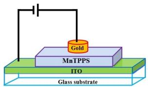
Fig. 3. Schematic representation of a switching device having configuration with active layer of MnTPPS and electrodes – ITO and gold [reprinted with permission from ref. 33].
