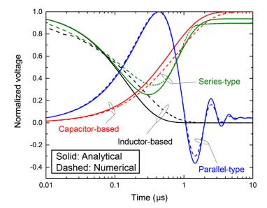
FIG. S1. Normalized voltages of inductor- and capacitor-based and parallel- and series-type waveform-selective metasurfaces using the same circuit constants ( $L = 100 \mu$ H, C = 1 nF,  $R_C = 10 k\Omega$ , and  $R_L = 10 \Omega$ ).
