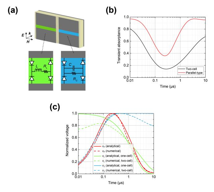
FIG. S3. (a) A two-cell model comprising a unit cell of an inductor-based waveform-selective metasurface and that of a capacitorbased waveform-selective metasurface. (b) Transient absorptances of the two-cell model and a parallel-type waveform-selective metasurface using the same circuit constants. (b) Their normalized voltages compared to those of individual inductor- and capacitorbased waveform-selective metasurfaces (indicated as "analytical, one-cell").
