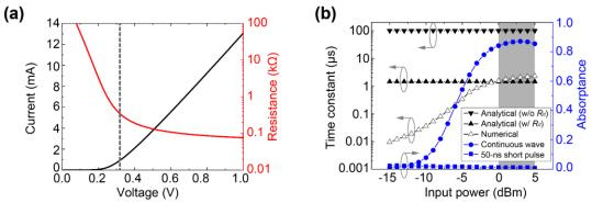
FIG. 4. (a) Relationship between the voltage and current of the diode used. The red solid curve and gray vertical line represent the effective diode resistance and the turn-on voltage, respectively. (b) Power dependence of the time constant of the inductor-based waveform-selective metasurface used in FIG. 2(a). The blue curves show the corresponding CW and short-pulse absorptances.
