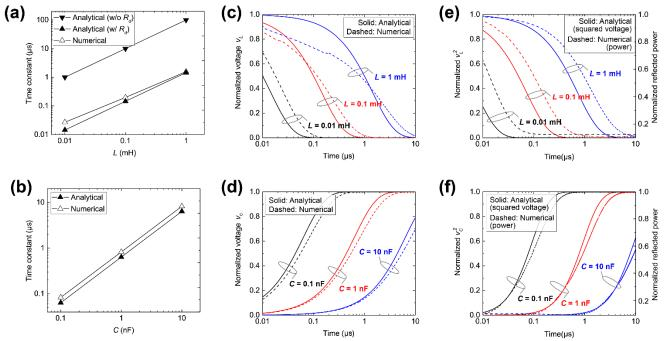
FIG. 2. Comparison in time constants of (a) an inductor-based waveform-selective metasurface and (b) a capacitor-based waveformselective metasurface. (c,d) Their inductor and capacitor voltages in the time domain. (e,f) Comparison with their reflected powers.
