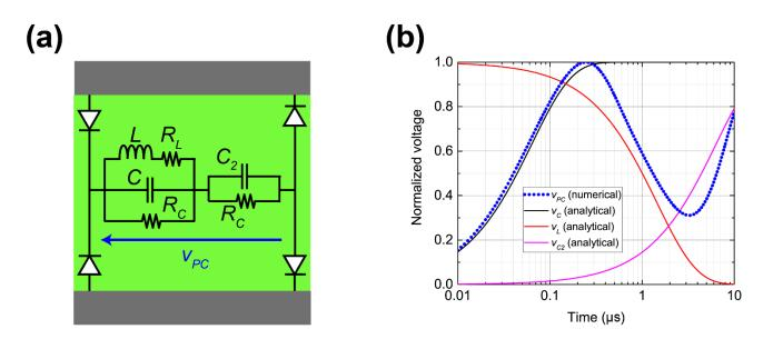
FIG. S2. (a) A structure integrating the circuit configuration of a parallel-type waveform-selective metasurface with that of a capacitor-based waveform-selective metasurface in series. (b) Its normalized voltage compared to those of individual waveform-selective metasurfaces.
