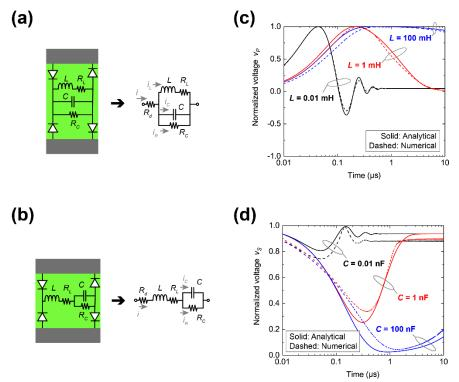
FIG. 3. (a,b) Circuit configurations used for a parallel-type and series-type waveform-selective metasurfaces and proposed equivalent circuit models. (c,d) Their time-domain voltages compared to simulation results.
