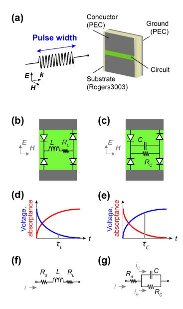
FIG. 1. (a) Pulse width and a periodic unit cell of a waveform-selective metasurface. (b,c) The circuit configurations deployed between patches for an inductor-based waveform-selective metasurface and a capacitor-based waveform-selective metasurface. (d,e) Their time-domain responses and (f,g) proposed equivalent circuit models that simplify the circuit response between patches.
