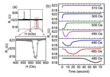
**FIG. 2.** (a) The longitudinal resistance (R<sub>xx</sub>) measurement with field scanning and magnified view of the MR peak for positive field scanning. (b) Magnetization relaxation curves in longitudinal Hall geometry at various perpendicular fields. The magnetization relaxation curve as a function of time mimics the R<sub>xx</sub> vs field curve indicates the domain wall motion with time.
