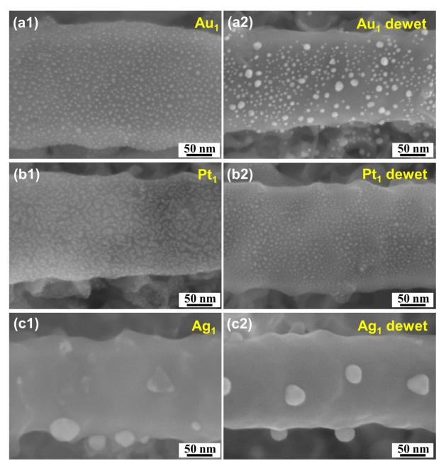
**Figure S4.** SEM images of TiO<sub>2</sub> nanotubes decorated with (a1,a2) 1 nm-thick Au; (b1,b2) 1 nm-thick Pt and (c1,c2) 1 nm-thick Ag. Samples (a2,b2,c2) were dewetted in Ar at 500 °C for 1 h.
