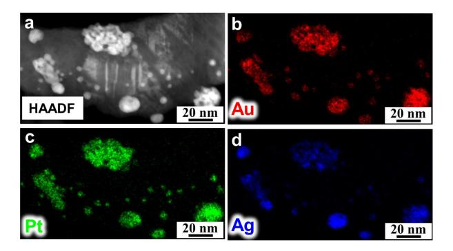
Figure S3. (a) HAADF image and (b-d) EDS mappings of TiO<sub>2</sub> nanotube after dealloying
