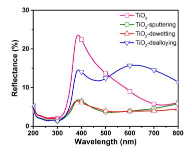
Figure S11. Reflectance measurements of TiO<sub>2</sub> NTs and Au<sub>1</sub>Pt<sub>1</sub>Ag<sub>6</sub>-decorated TiO<sub>2</sub> NTs.
