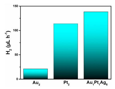
**Figure S8.** Photocatalytic H<sub>2</sub> generation of TiO<sub>2</sub> NTs decorated with 2 nm Au (Au2), 2 nm Pt (Pt2) and porous AuPt alloy particles (Au1Pt1Ag6). After sputtering, plain Au and Pt decorated TiO<sub>2</sub> tubes were annealed at 500 °C in Ar to induce dewetting.
