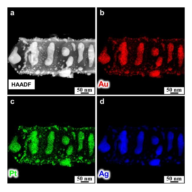
**Figure S2.** (a) HAADF image and (b-d) EDS mappings of TiO<sub>2</sub> nanotube after dewetting Au<sub>1</sub>Pt<sub>1</sub>Ag<sub>6</sub>. Homogeneous AuPtAg alloyed nanoparticles are formed on the tube wall.
