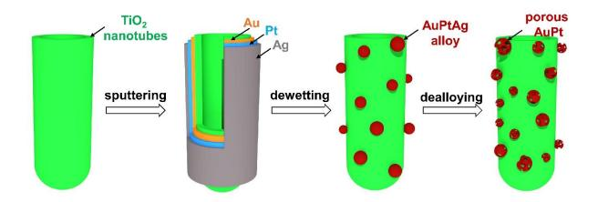
Scheme 1. Formation of porous AuPt alloyed NPs on  $TiO_2$  NTs. Noble metal was deposited on  $TiO_2$  NTs by a plasma sputtering machine. Dewetting was carried out by a thermal treatment in Ar and dealloying was conducted by selective chemical dissolution in nitric acid.
