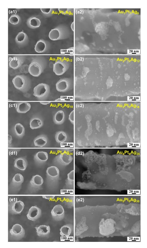
**Figure S7.** SEM images of porous AuPt alloy-nanoparticle-decorated TiO<sub>2</sub> nanotubes: (a1,a2) 1 nm-thick Au, 1 nm-thick Pt and 6 nm-thick Ag; (b1,b2) 2 nm-thick Au, 2 nm-thick Pt and 12 nm-thick Ag; (c1,c2) 3 nm-thick Au, 3 nm-thick Pt and 18 nm-thick Ag; (d1,d2) 4 nm-thick Au, 4 nm-thick Pt and 24 nm-thick Ag; (e1,e2) 5 nm-thick Au, 5 nm-thick Pt and 30 nm-thick Ag. All samples were dewetted in Ar at 500 °C for 1 h, followed by a dealloying step in HNO<sub>3</sub> at 25 °C for 4 h.
