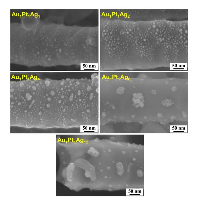
**Figure S6.** SEM images of porous AuPt alloy-nanoparticle-decorated  $TiO_2$  nanotubes. All samples were sputtered with 1 nm-thick Au, 1 nm-thick Pt and different amounts of Ag (1, 2, 4, 6 and 12 nm-thick). The samples then were dewetted in Ar at 500 °C for 1 h, followed by a dealloying step in HNO<sub>3</sub> at 25 °C for 4 h.
