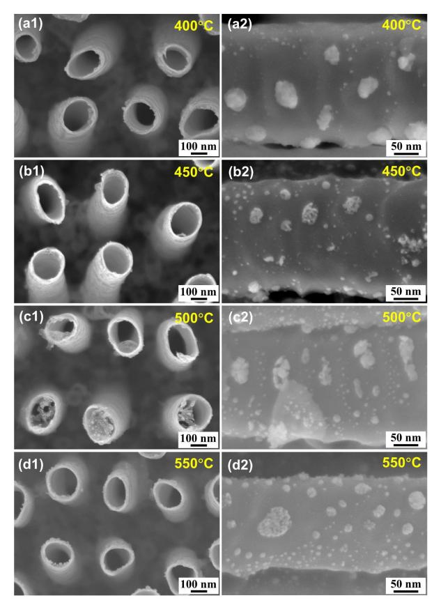
**Figure S9.** SEM images of TiO<sub>2</sub> nanotubes decorated with 1 nm-thick Au, 1 nm-thick Pt and 6 nm-thick Ag followed by a thermal dewetting in Ar for 1 h at different temperatures (a1,a2) 400 °C, (b1,b2) 450 °C, (c1,c2) 500 °C and (d1,d2) 550 °C. All samples were dealloyed in HNO<sub>3</sub> at 25 °C for 4 h.
