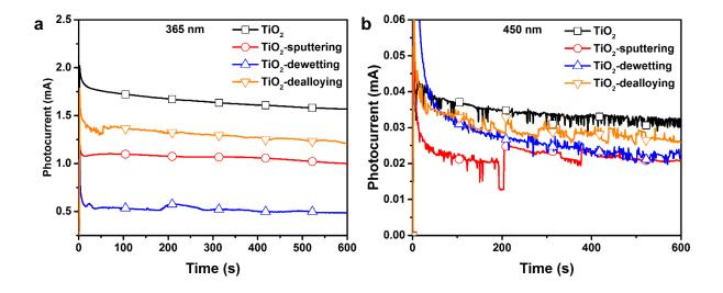
**Figure S12.** Photocurrent measurements of  $TiO_2$  nanotubes and Au1Pt1Ag6-decorated  $TiO_2$  NTs using a light source of: (a) 365 nm and (b) 450 nm.
