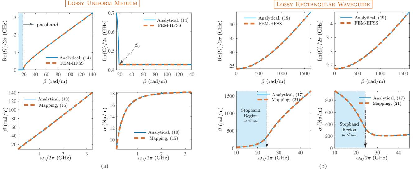
FIG. 2. The complex eigenmodes  $\Omega(\beta)$  and the mapped frequency dependent complex propagation constants for the case of (a) Lossy Bulk Medium with  $\epsilon_r = 4.2$  and  $\sigma_e = 0.2$  S/m, and (b) Lossy rectangular waveguides with  $\epsilon_r = 4.2$ ,  $\delta = 0.2$ , and  $a = 3$  mm.
