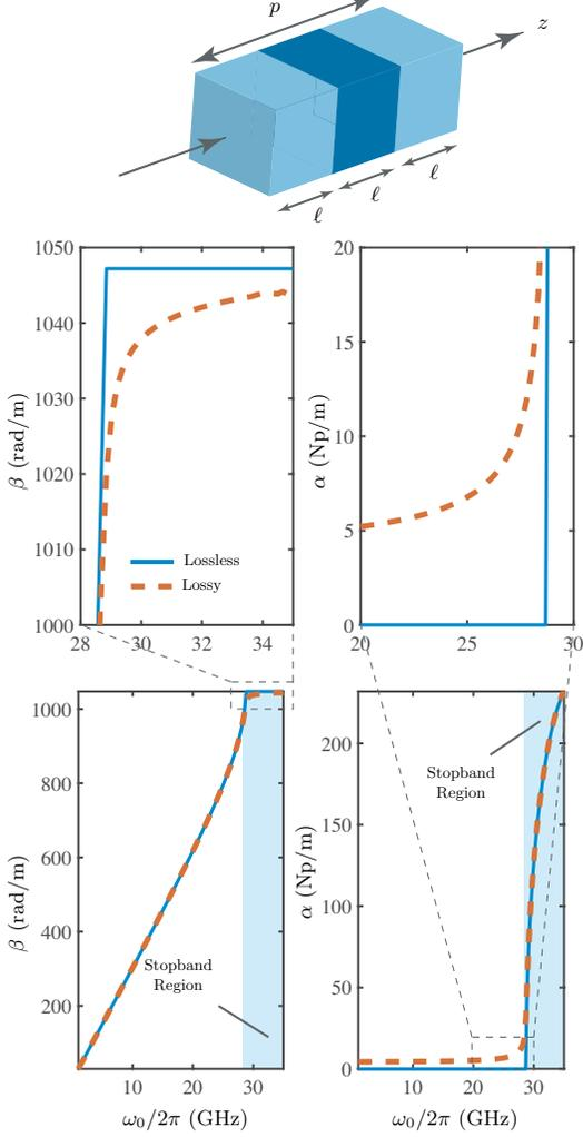
FIG. 5. The analytical complex propagation constant  $\gamma$  of a periodic dielectric stack under lossy and lossless conditions. Design parameters are:  $\ell = 1$  mm; Outer slabs: air; Inner slab:  $\epsilon_r = 4.2$  and  $\sigma_e = 0$  S/m for lossless and  $\sigma_e = 0.1$  S/m for lossy case.
