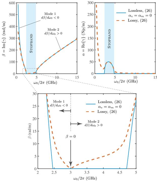
FIG. 3. The analytical complex propagation constant  $\gamma$  of a Drude dispersive metamaterial under lossy and lossless conditions. Design parameters are:  $\omega_{ep} = 15$  Grad/s,  $\omega_{mp} = 30$  Grad/s and  $\alpha_e = \alpha_m = 2 \times 10^9$ .
