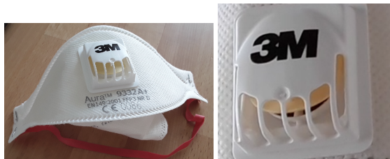
Fig. 20. Left: FFP3-mask with one-way valve; right: during exhaling, the one-way-valve (yellow) opens and humid air leaves the mask unfiltered
