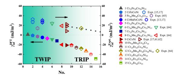
**Figure 3.** Correlation between the calculated SFEs ( $\gamma_{isf}^{DFT}$ , filled and half-filled symbols) and the observed strengthening mechanisms (TWIP/TRIP) [61, 64, 109-111] in a group of MEAs and HEAs. Available experimental SFEs ( $\gamma_{isf}^{Expt.}$ , empty symbols) are also plotted for comparison. Experimental SFEs for TRIP alloys are usually not available but should approach zero as indicated by the dashed line according to the experimental
